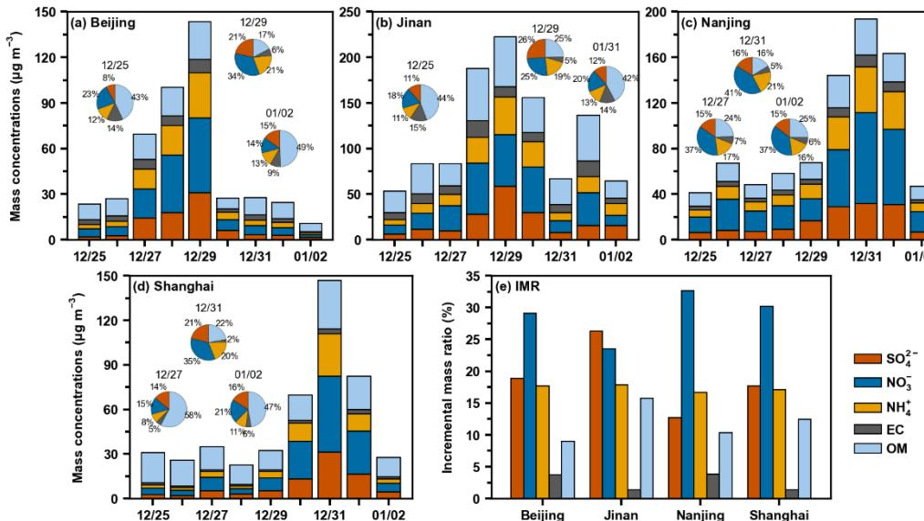
**Figure R3-1.** Mass concentrations and fractions (a–d) and incremental mass ratio (e) of the major PM<sub>2.5</sub> chemical compositions ( $\text{SO}_4^{2-}$ ,  $\text{NO}_3^-$ ,  $\text{NH}_4^+$ , EC, and OM) in Beijing, Jinan, Nanjing, and Shanghai.
