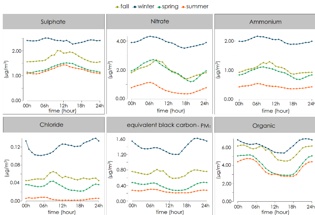
Fig. 3: Seasonal diurnal cycle of PM 1 for ACSM organic and inorganic species (Time is in UTC).
