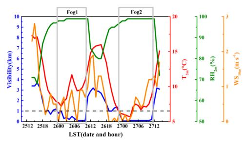
**Figure 1.** Time series of visibility, 2 m temperature  $(T_{2m})$ , 2 m relative humidity  $(RH_{2m})$ , and 10 m wind speed  $(WS_{10m})$  above the ground at the Nanjing observation site  $(31.93^{\circ}N, 118.9^{\circ}E)$ . Fog1 and Fog2 in the light grey box are the two fog events. Time '2512' indicates 12:00 local standard time (LST) (LST = Universal Time Coordinated + 8 h) on 25 November 2018. The other time expressions follow the same logic.
