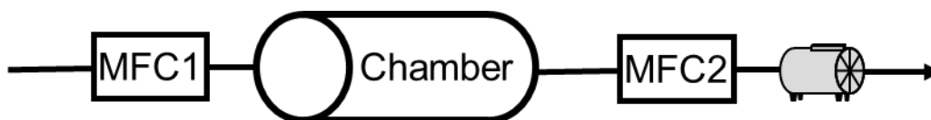
189 190 191 Figure S14. Schematic diagram for investigating the airtightness of the reaction and reference chambers, 192 where MFC1 could measure air flow rate and pressure at the chamber inlet, MFC2 could measure air flow 193 rate and pressure at the chamber outlet.
