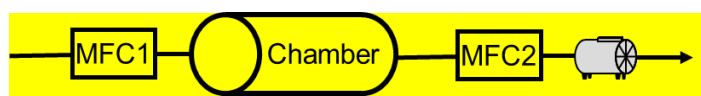
Figure S14. Schematic diagram for investigating the airtightness of the reaction and reference chambers, where MFC1 could measure air flow rate and pressure at the chamber inlet, MFC2 could measure air flow rate and pressure at the chamber outlet.”
