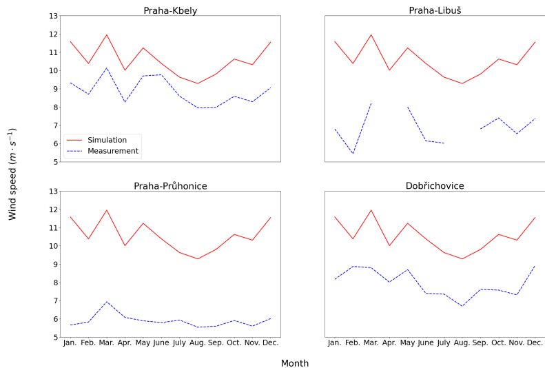
Figure 16. Annual cycle of monthly averaged maximum daily wind-speeds from model simulation (red) and observations from four station in/around Prague (red); averaging is done for days when the daily PM10 model bias is larger than 50 \mu\text{g m}^{-3} .
