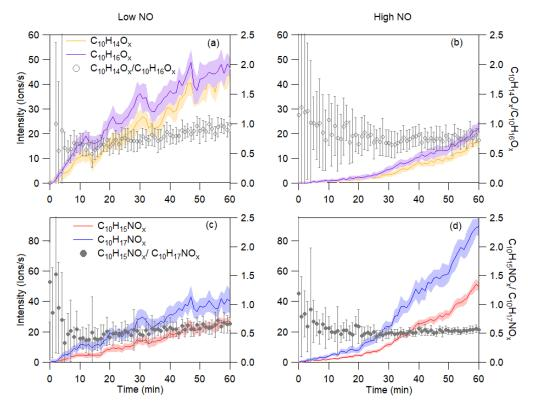
Figure 4. Time series of C<sub>10</sub>H<sub>15</sub>O<sub>x</sub>• and C<sub>10</sub>H<sub>17</sub>O<sub>x</sub>• related families of carbonyls and organic nitrates during the first 60 min of the experiments. The carbonyl families C<sub>10</sub>H<sub>14</sub>O<sub>x</sub> (yellow), C<sub>10</sub>H<sub>16</sub>O<sub>x</sub> (purple), and their concentration ratio (C<sub>10</sub>H<sub>14</sub>O<sub>x</sub> / C<sub>10</sub>H<sub>16</sub>O<sub>x</sub>) are shown for (a) low and
