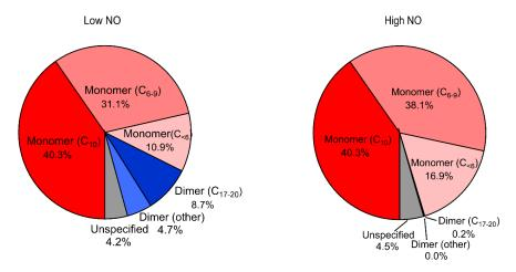
Figure 2. HOM product distribution including monomers (C<sub>10</sub>, C<sub>6-9</sub>, C<sub><6</sub>), dimers (C<sub>17</sub>-C<sub>20</sub>, other), and unspecified species in low and high NO conditions.
