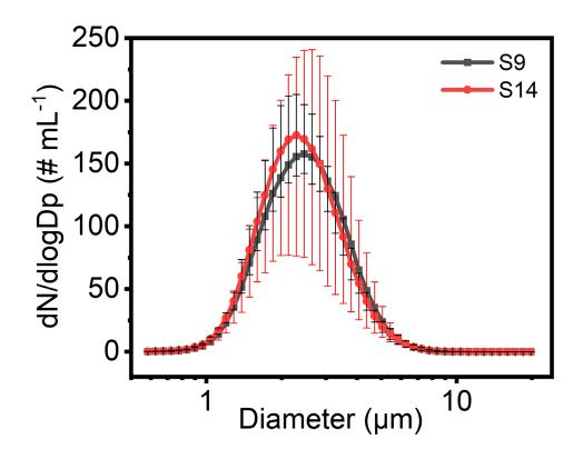
**This study:** Supplementary Figure S8. Particle size distribution of dust aerosols produced from soil S9 and S14. The size distribution was detected by an Aerodynamic Particle Sizer (APS), which size range is 0.5-20 μm.
