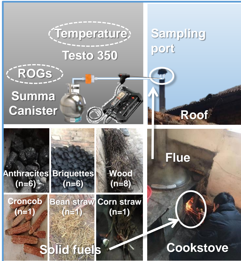
Figure S1. Sampling diagram relates to six solid fuels types, household stoves, sampling port and equipment. n refers to the number of different samples.
