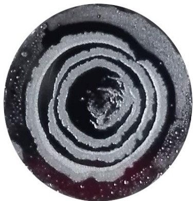
Figure 6: A photograph of the cooling stage of the ESEM covered with the crystallized CsCl salt after the sublimation of the 0.5 M non-seeded sample at -20\text{ }^{\circ}\text{C} . The diameter of the stage is about 6 mm. The pattern of the concentric circle is nicely visible.
