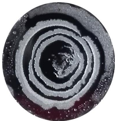
835 Figure 6: A photograph of the cooling stage of the ESEM covered with the crystallized CsCl salt after the sublimation of the 0.5 M non-seeded sample at -20\text{ }^{\circ}\text{C} . The diameter of the stage is about 6 mm. The pattern of the concentric circle is nicely visible.
