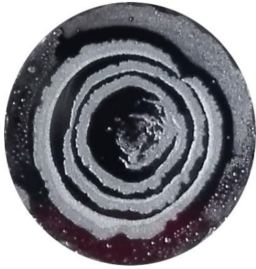
Figure 6: A photograph of the cooling stage of the ESEM covered with the crystallized CsCl salt after the sublimation of the 0.5 M non-seeded sample at -20\text{ }^{\circ}\text{C} . The diameter of the stage is about 6 mm. The pattern of the concentric circle circles is nicely visible.
