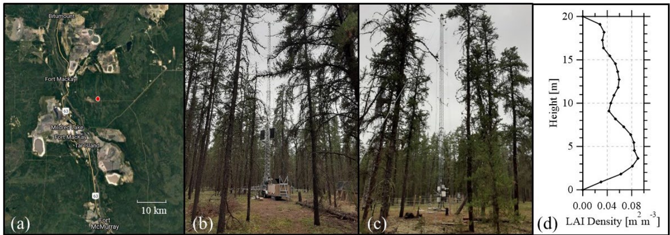
Figure 1: (a) The study area and surrounding location showing the location of the towers (red dot) relative to oil sands mining and production facilities. (b) A photo of YAJP tower. (c) A photo of WBEA 1004 tower. (d) The LAI density profile near the YAJP station. Map image is © Google Maps. Photos taken by authors.
