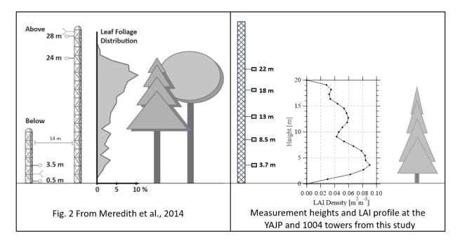
This figure (not included in the revised manuscript) compares the above-canopy measurement locations and LAI from Meredith et al. (2014) with the measurement heights and LAI from this study, demonstrating that the two highest measurement heights can be considered "above-canopy" relative to the forest leaf distribution.
