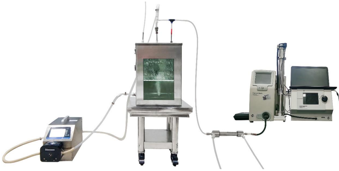
14 Figure S2. The physical drawing of a plunging jet-sea spray aerosol generator.
