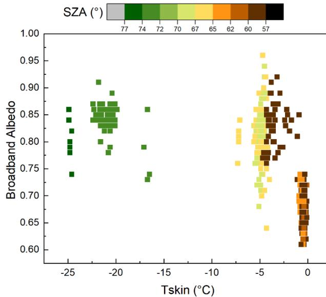
Figure 2: Broadband surface albedo measured during AFLUX and ALOUD as a function of solar zenith angle (SZA) and skin temperature ( $T_{skin}$ ). The data are limited to cloud-free conditions and sea ice coverage larger than 99 %.
