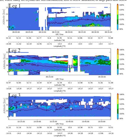
Figure 4: The three panels show the RHi from Fig. 3 in more detail. The black contour represents the cloud edge. White areas are due to lack of measurements in these regions, because of detector saturation.
