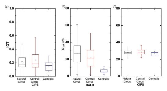
Figure 9: Box charts of (a) IOT from satellite observations by CiPS, (b) R<sub>eff</sub> from HALO in situ measurements, and (c) from CiPS. Each bar contains the information of the maximum, minimum, interquartile range (25% percentile to 75% percentile), median (horizontal line) and mean (square).
