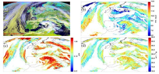
Figure 1: (a) The false color RGB image from MSG/SEVIRI on 26 March 2014 at 10:45 UTC showing Europe and the Eastern part of the North Atlantic Ocean, (b) corresponding ice clouds CTH, (c) IOT and (d) R<sub>eff</sub> from CiPS
