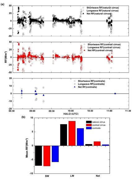
670 Figure 12: (a) TOA LW, SW and net RF of natural cirrus, contrail cirrus and contrails from our RTM simulations for HALO probed ice particles along the HALO flight path over NAR on 26 March 2014, and(b) corresponding mean values.
