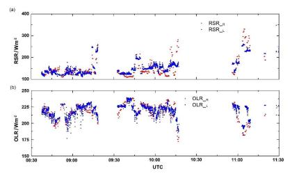
Figure 11: TOA RSR and OLR from our RTM simulations (RSR\_L, OLR\_L) for probed ice particles and RRUMS algorithm results (RSR\_R, OLR\_R) for single SEVIRI pixel along the HALO flight path. All simulations are plotted here.
