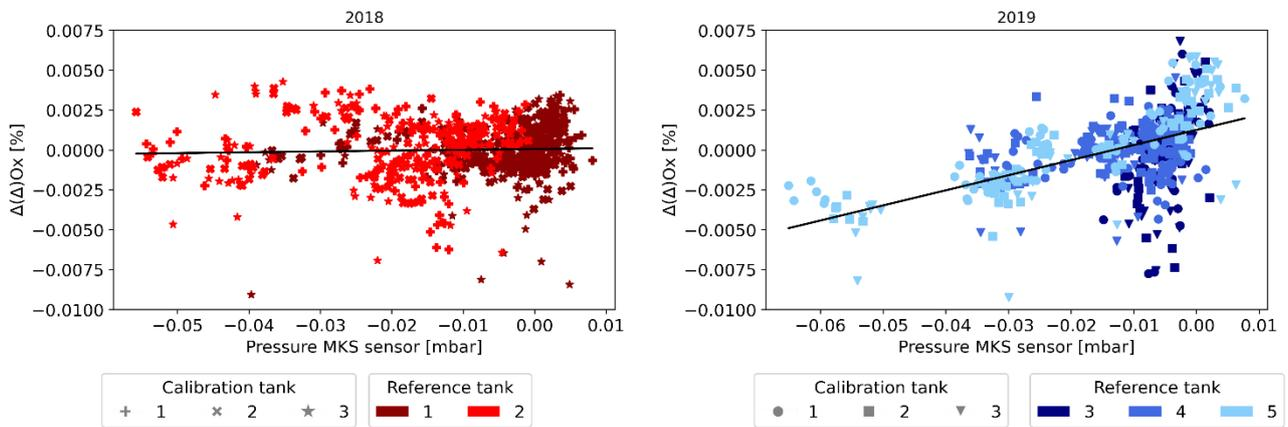
Figure 1 The relationship between the differential pressure measured by the MKS sensor and the 4 minute  $\Delta(\Delta)O_2$  values of the calibration tank values during the 2018 and 2019 measurement period. The  $\Delta(\Delta)O_2$  values are the deviations from the mean of the specific calibration tank.
