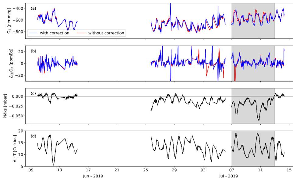
Figure 2 The corrected and not corrected 30-minute averaged O<sub>2</sub> concentrations at 23 m for the PMKS deviations (a), together with the corrected and not corrected gradient of O<sub>2</sub> (b). The time series for the 2019 measurement period of the PMKS (c) and the air temperature (d). Same as Figure B1 in the appendix.
