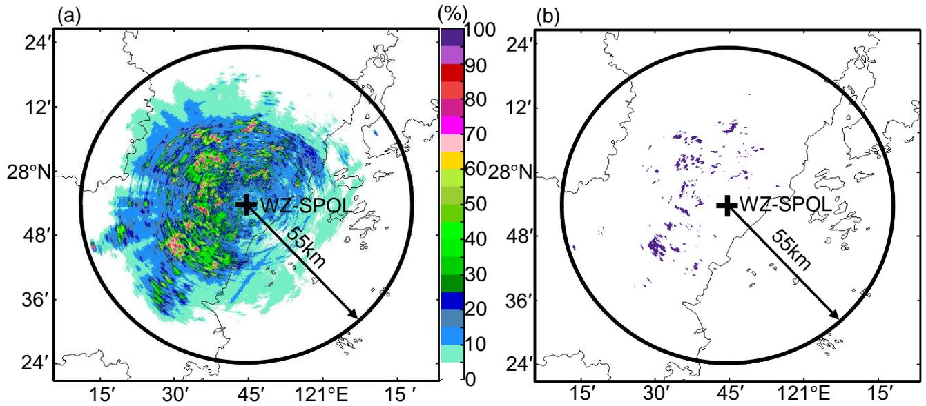
810 Fig. 3. (a) Statistics of pixels with  $Z_H > 0$  dBZ within 55 km from the WZ-SPOL radar; (b) residual static ground clutter mask of the WZ-SPOL radar.
