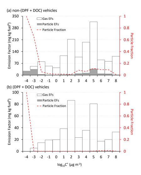
Figure 7. The emission factors of gaseous and particulate I/SVOCs (hollow and filled stack columns) and the particle mass fraction (red dashed line) in each volatility bin computed from (a) non-(DPF + DOC) vehicles and (b) (DPF + DOC) vehicles.
