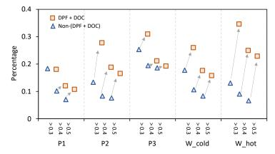
Figure 5. The increment of I/SVOC with O:C > 0.3, 0.4, and 0.5 from non-(DPF + DOC) to (DPF + DOC) vehicles under low-speed stage (P1), middle-speed stage (P2), high-speed stage (P3), and whole (W\_cold, W\_cold) driving cycles.
