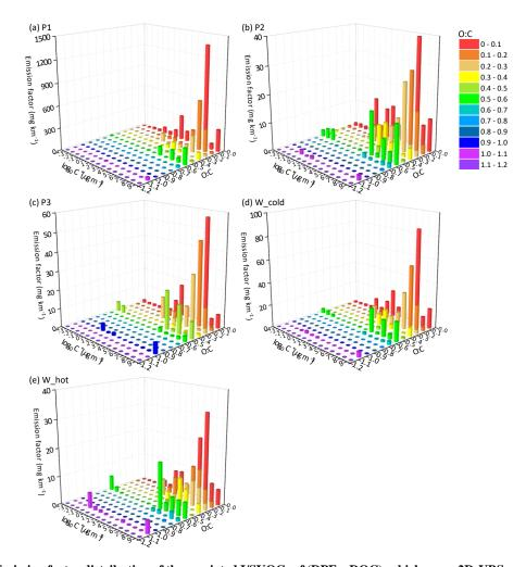
Figure 4. Emission factor distribution of the speciated I/SVOCs of (DPF + DOC) vehicles on a 2D-VBS space of (a) low-speed stage (P1), (b) middle-speed stage (P2), (c) high-speed stage (P3), (d) whole (W\_cold), and whole (W\_hot) driving cycles. Different colours indicate different O:C ratios segmented into 12 bins: 0-0.1, 0.1-0.2, 0.2-0.3, 0.3-0.4, 0.4-0.5, 0.5-0.6, 0.6-0.7, 0.7-0.8, 0.8-0.9, 0.9-1.0, and 1.1-1.2.
