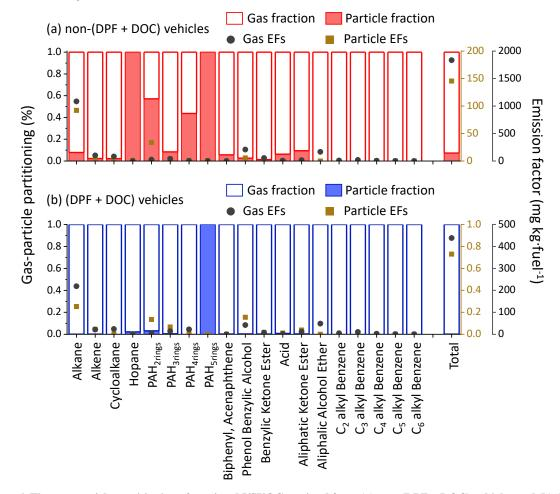
Figure 6. The gas-particle partitioning of speciated I/SVOCs emitted from (a) non-(DPF + DOC) vehicles and (b) (DPF + DOC) vehicles. The hollow and filled columns represent the gas and particle fraction, respectively. The grey dots and brown squares represent the emission factors of the gaseous and particulate I/SVOCs.
