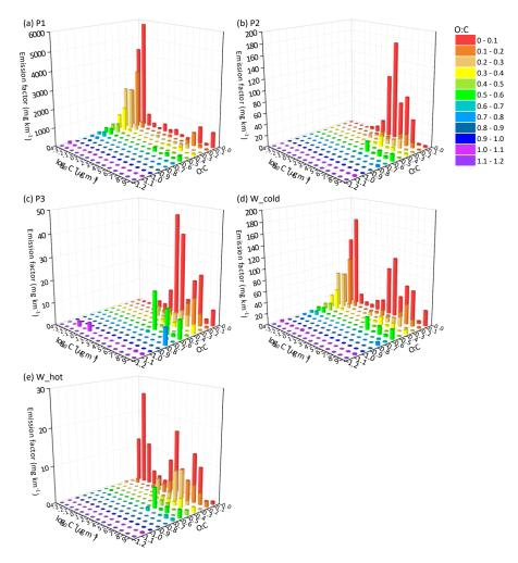
Figure 3. Emission factor distribution of the speciated I/SVOCs of non-(DPF + DOC) vehicles on a 2D-VBS space of (a) low-speed stage (P1), (b) middle-speed stage (P2), (c) high-speed stage (P3), (d) whole (W\_cold), and whole (W\_hot) driving cycles. Different colours indicate different O:C ratios segmented into 12 bins: 0-0.1, 0.1-0.2, 0.2-0.3, 0.3-0.4, 0.4-0.5, 0.5-0.6, 0.6-0.7, 0.7-0.8, 0.8-0.9, 0.9-1.0, and 1.1-1.2.
