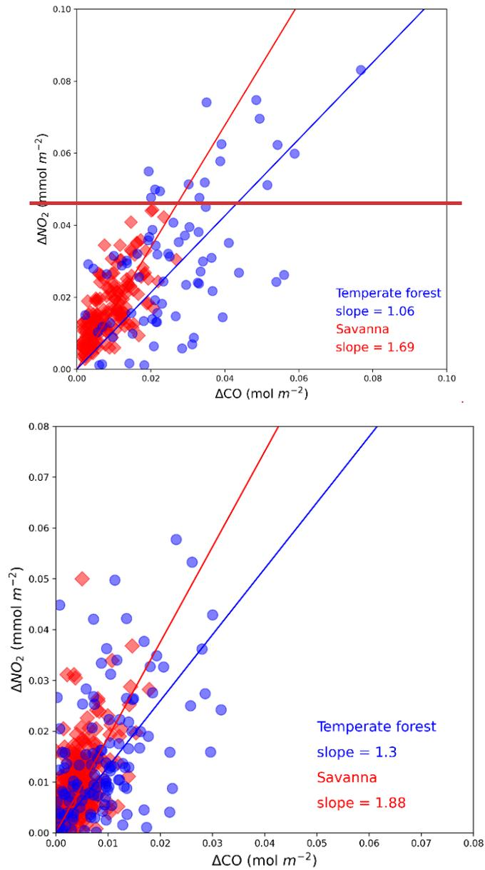
Figure 7: The relationship between daily  $\Delta\text{CO}$  ( $\text{mol m}^{-2}$ ) and daily  $\Delta\text{NO}_2$  ( $\text{mmol m}^{-2}$ ) was derived from TROPOMI for all regions. The slope of linear fit with an intercept at zero represents the combustion efficiency of different fire types.
