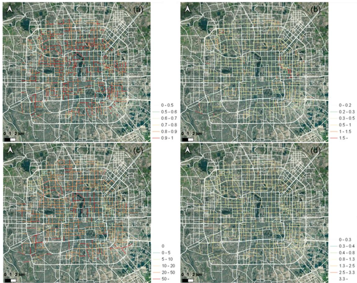
Figure S1. Spatial distribution of street canyon geometry in Beijing (© Microsoft). (a) Length of actual street canyon to the total street length, (b) Height to width ratio, (c) Length to height ratio and (d) Height symmetrical ratio.
