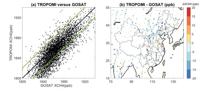
**Figure 2**. Comparison between 2019 TROPOMI and GOSAT observations of XCH<sub>4</sub> over East Asia. (a) Scatter plot of daily observations on the GEOS-Chem  $0.25^{\circ} \times 0.3125^{\circ}$  grid. Green lines indicate absolute TROPOMI-GOSAT differences of 20 ppb and we exclude the outlying TROPOMI observations. (b) Spatial pattern of annual mean differences  $\Delta$ XCH<sub>4</sub> between TROPOMI and GOSAT observations after outlying TROPOMI data have been excluded. The
