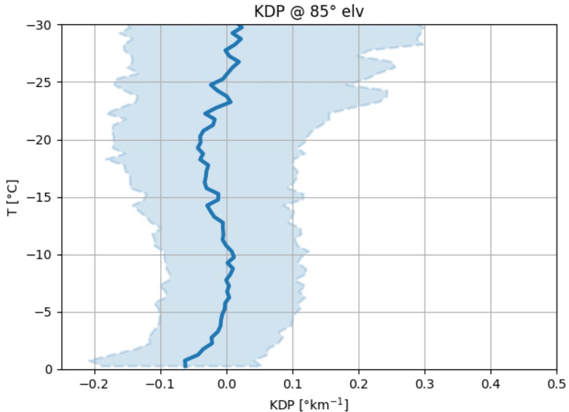
Figure 1: median KDP (solid line) and quantiles (shading) of KDP calculated from PPI at 85° elevation
