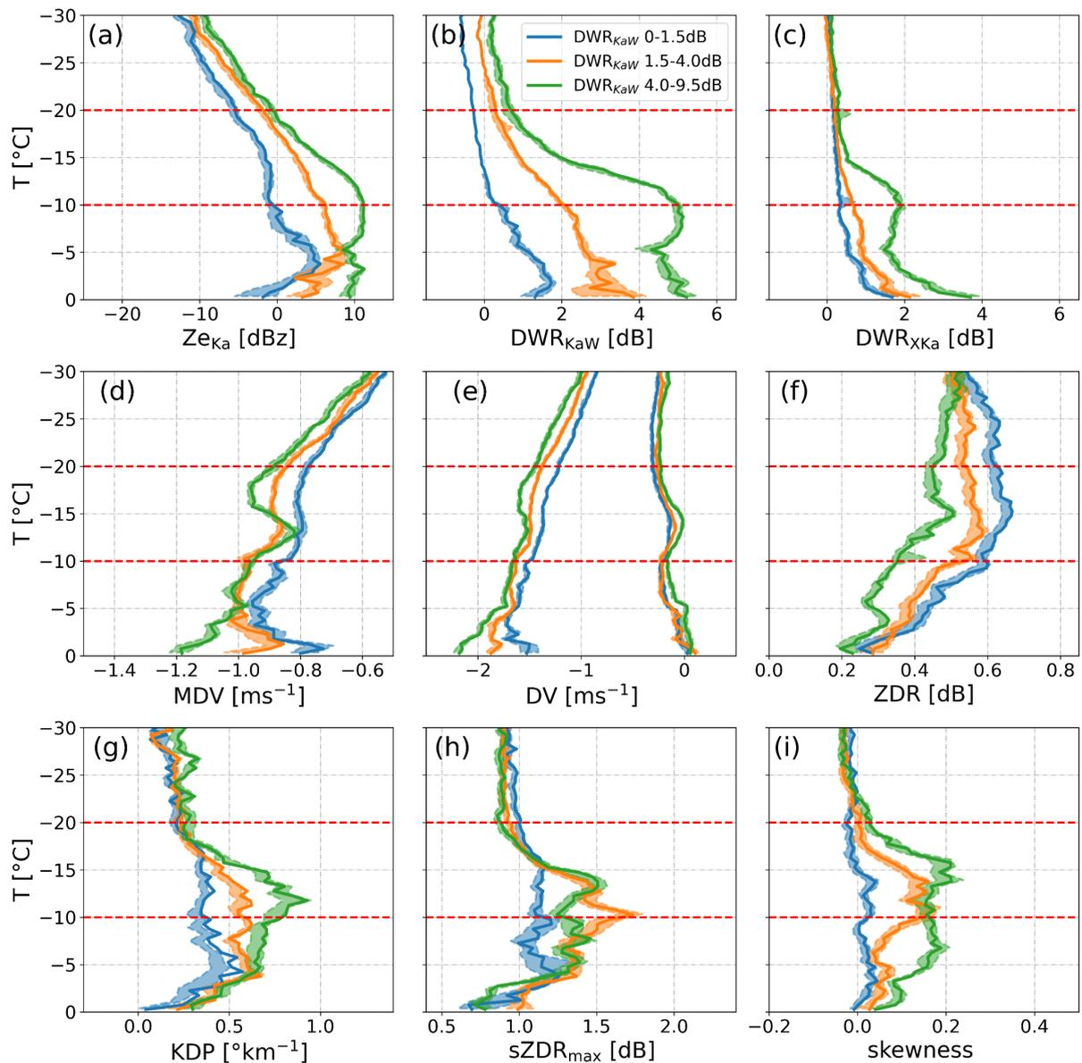
Figure 3: bootstrapping analysis of the DWR-statistics: distribution of medians of 50 subsamples. The subsample size was 50% of the original dataset. The shaded areas indicate the 25 and 75 percentile of the distribution of medians. The solid line is the median of the original dataset.
