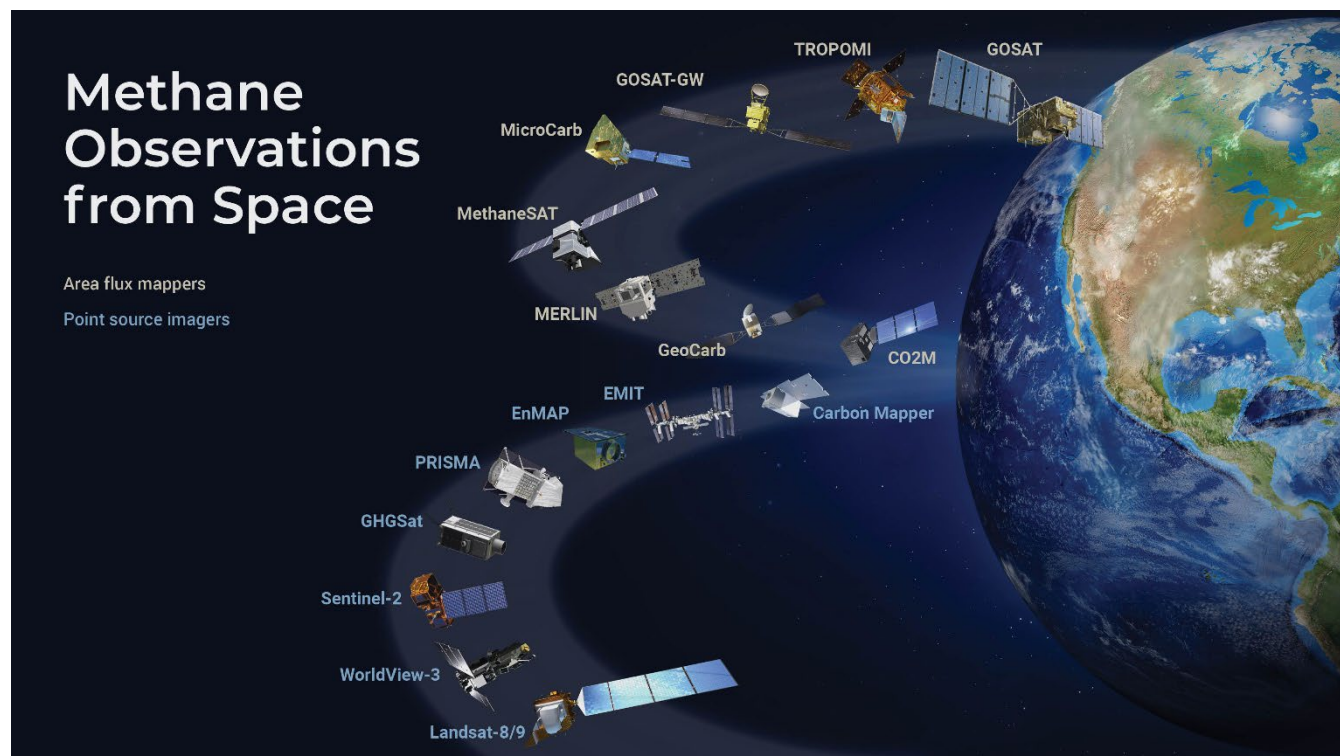
Figure 1: Satellite instruments for observation of methane in the shortwave infrared (SWIR). Area flux mappers are designed to quantify total methane emissions on regional to global scales. Point source imagers are designed to quantify emissions from individual point sources by imaging the atmospheric plumes. Satellite icons were obtained from https://www.gosat.nies.go.jp for GOSAT; https://directory.eoportal.org for PRISMA and WorldView-3; Wikipedia Commons for TROPOMI, EMIT (International Space Station), and Sentinel-2; https://space.skyrocket.de for GOSAT-GW, MERLIN, CO2M, and Carbon Mapper; https://microcarb.cnes.fr for MicroCarb; https://www.methanesat.org for MethaneSAT; https://www.ou.edu/geocarb/mission for GeoCarb; https://www.planetek.it/ for PRISMA; https://www.ghgsat.com/ for GHGSat; https://www.enmap.org/mission for EnMAP; and https://www.usgs.gov/landsat-missions for Landsat-8/9.
