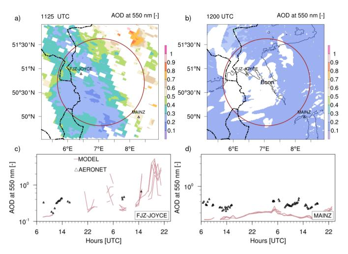
**Figure 3.** a-b) Satellite and model estimate of aerosol optical depth (AOD at 550 nm) over the Bonn Radar domain on 2015 4 July. The two available AERONET stations over the Bonn Radar domain is also shown. c-d) Time-series of measured and simulated ensemble AOD over FJZ-JOYCE and MAINZ AERONET station.
