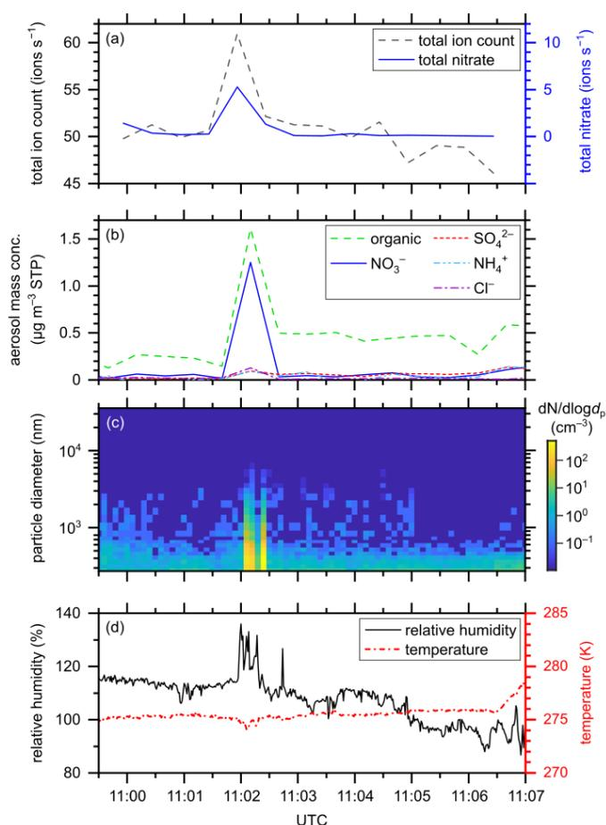
350 **Figure 4:** Gas-phase and particle-phase parameters during the API measurement on flight segment 06.2 on 04 June 2020 above the
