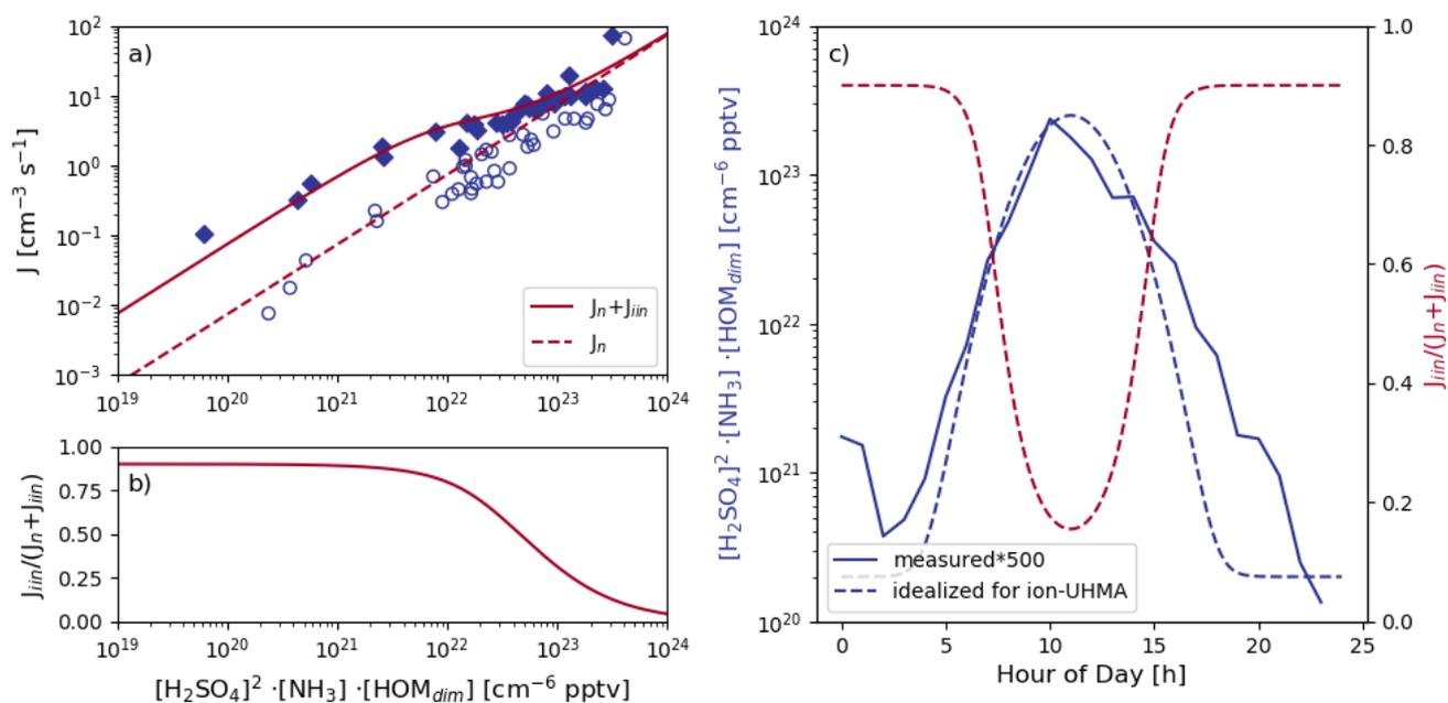
**Figure 5:** The importance of ion-induced nucleation in the boreal forest. a) shows the measured nucleation rates (diamonds under galactic cosmic ray conditions and circles under neutral conditions) and the parametrizations (Eq. (2) and Eq. (4)). b) shows the fraction of ion-induced nucleation from total nucleation rate against the parametrizations from Eq. (2) and Eq. (4). c) shows the diurnal pattern of the calculated nucleation rates and ion-induced fraction in Hyytiälä.
