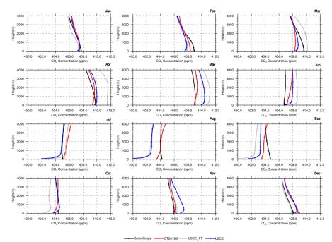
Figure 3: Comparison of average monthly vertical profiles of CO<sub>2</sub> concentration from global atmospheric transport models over the model domain during daytime (11:30 to 16:30 local time) in 2017. Panels show data for respective months as indicated on the top of each panel.
