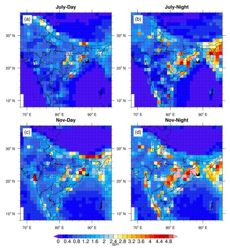
Figure 4: Monthly averaged values of representation error estimated for surface CO<sub>2</sub> concentration (second model level, mean height is ~200 m from sea level) over the region 8° N to 37° N and 68° E to 96° E during 2017. a) July daytime (11:30 to 16:30 local time) b) July nighttime (23:30 to 4:30 local time). c) November daytime. d) November nighttime.
