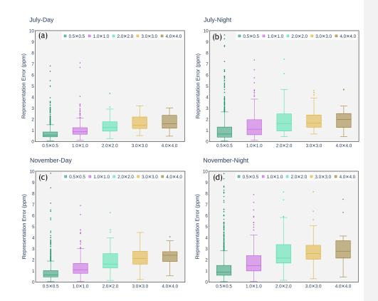
1310 Figure 7: Variability of derived surface representation error over India for different horizontal resolutions. Boxes indicate the central 50%, the bar across the box is median value, and the whiskers indicate the value between 5 and 95 percentiles. Individual data points shown are the outliers. a) Representation error estimated for July daytime. b) July nighttime. c) November daytime. d) November nighttime.
