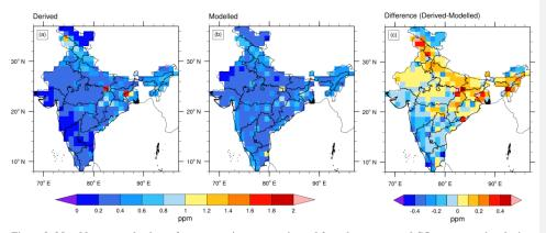
Figure 9: Monthly averaged values of representation error estimated for column averaged CO<sub>2</sub> concentration during July daytime (11:30 to 16:30 local time) in 2017. a) Representation error derived from WRF-GHG simulations as explained in Sect. 2.3. b) Representation error calculated from the multivariate linear model as described in Sect. 3.5. c) Difference between (a) and (b).
