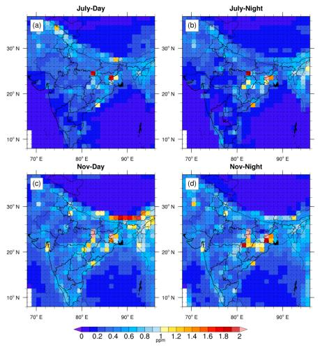
Figure 5: Monthly averaged values of representation error estimated for column averaged CO<sub>2</sub> concentration over the region 8° N to 37° N and 68° E to 96° E during 2017. a) July daytime (11:30 to 16:30 local time) b) July nighttime (23:30 to 4:30 local time). c) November daytime. d) November nighttime.
