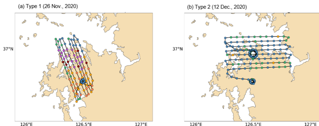
Figure 2. Flight tracks for two Cessna Grand Caravan 208 B aircraft over Pandora sites (left) PA 4 and (right) PA 1 during the GMAP-2020 campaign. Colored circles indicate airborne NO 2 concentration observations. Stacked circles indicate spiral flights conducted over two sites.
