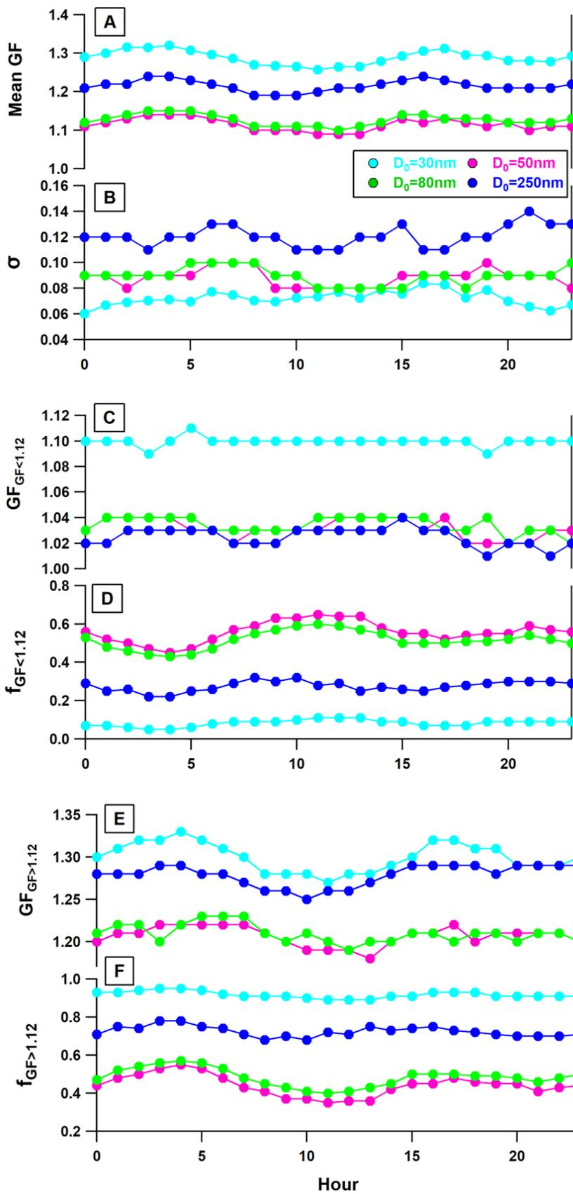
**Figure 7** Diurnal variation of A) mean GF, measured at RH=90% , B) standard deviation of the mean GF, C) GF of non or slightly hygroscopic particles, D) the number fraction of non or slightly hygroscopic particles, E) GF of moderately hygroscopic particles, and F) the number fraction of moderately hygroscopic particles
