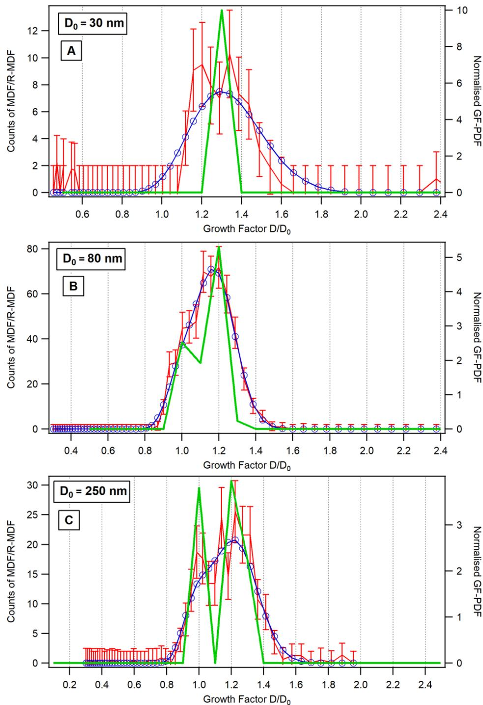
**Figure 3** Example of growth factor distributions measured at RH=90% of  $D_0=30$ nm particles (Panel (A), internally mixed), of  $D_0=80$ nm particles (Panel (B), continuum of mixing states) and of  $D_0=250$ nm particles (Panel (C), externally mixed with distinct modes). The red line
