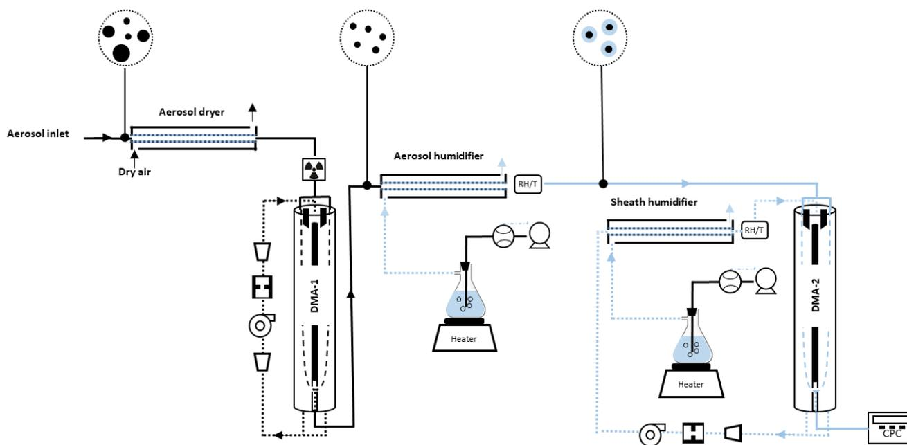
100 **Figure 2** Schematic diagram of the HTDMA system
