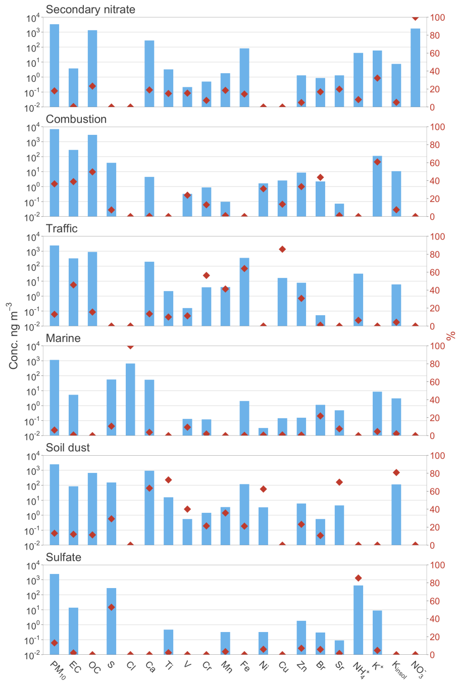
Figure 8. Chemical profiles of the factors obtained by PMF analysis, showing the mass contribution in \text{ng m}^{-3} of each species within each source (blue bars) and the average percentage contribution of each source to the total concentration of each element (red points)
