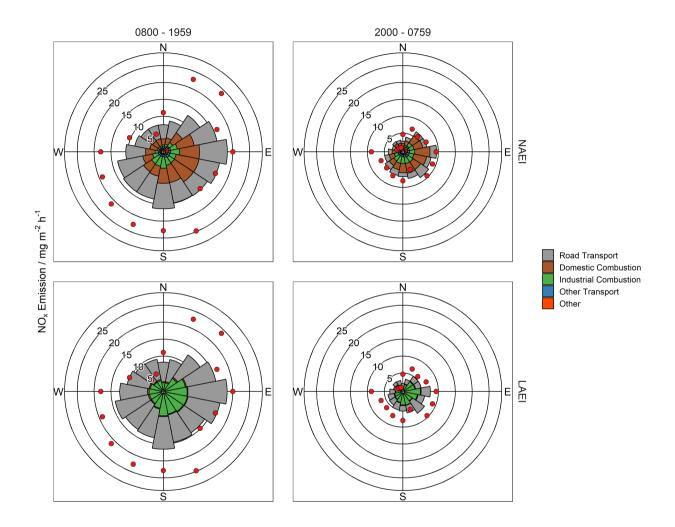
**Figure 11.** NO<sub>x</sub> emissions (red) measured at the BT Tower March - July 2017 and the NAEI's estimated emission (bars) from within the flux footprint, averaged by 22.5  $^{\circ}$  wind sector bins. NAEI emissions are coloured by source sector contribution. The left hand panel shows all data between 0800 - 1959 and the right hand panel shows all data between 2000 - 0759.
