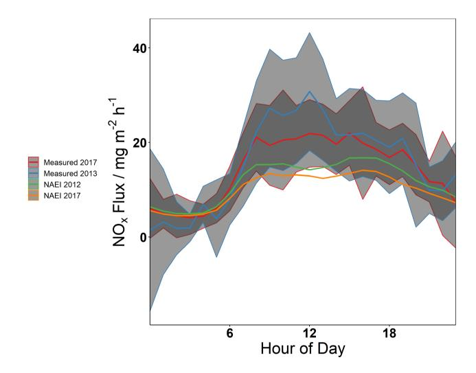
**Figure 13.** Diurnal profiles of measured NO<sub>x</sub> flux in 2013 (blue, recalculated from Lee et al. (2015)) and blue (this study compared with inventory time series generated from 2012 (green) and 2017 (orange) versions of the NAEI.
