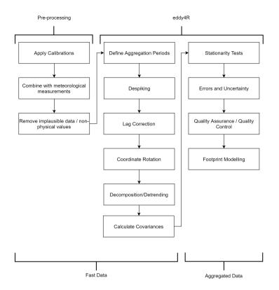
Figure A1. Schematic eddy covariance calculation workflow.
