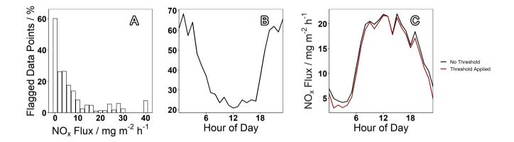
**Figure 4.** A - Percentage of flux records flagged by quality control routines in 2 mg m<sup>-2</sup> h<sup>-1</sup> bins. B - Percentage of flux records flagged by quality control routines by hour of day. C - NO<sub>x</sub> flux diurnal cycle where black has had all records flagged by quality control routines removed and red has only had them removed if the flux magnitude was also greater than 5 mg m<sup>-2</sup> h<sup>-1</sup>
