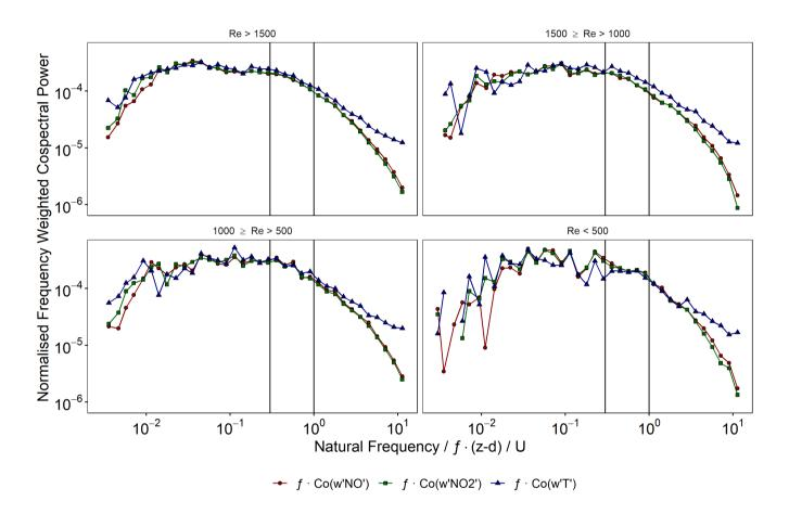
**Figure 6.** Normalised co-spectra of vertical wind with NO (red, circle),  $NO_2$  (green, square) and temperature (dark blue, triangle). Co-spectra are grouped by main sample line Reynolds number. Vertical bars mark 0.3 Hz and 1 Hz where data at frequencies greater than these have been used to derive the correction factors presented in table 1
