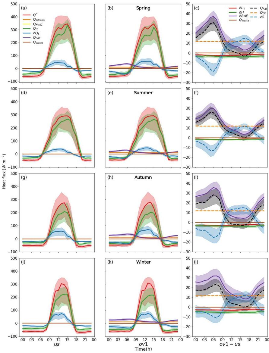
524 Figure B1. As Figure 1, but uses *ov1* for occupied building case in (b, e, h, k) and the heat flux difference with respect to
