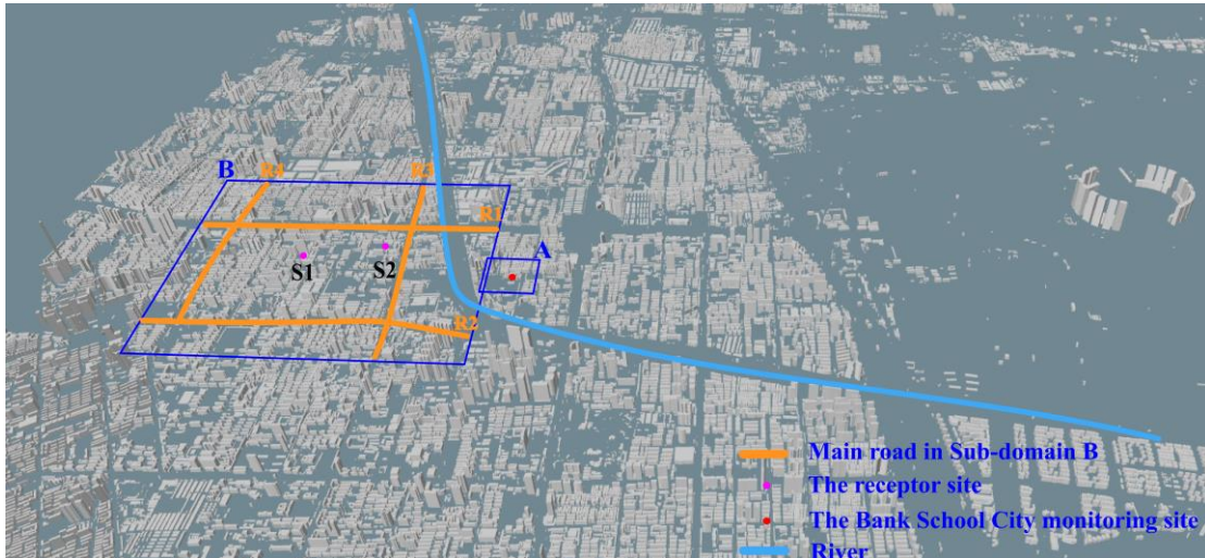
Figure R4: The computational domain of the CFD model, with magenta dots (S1 and S2) indicating the receptor sites and Orange line indicating the main roads in Sub-domain B.
