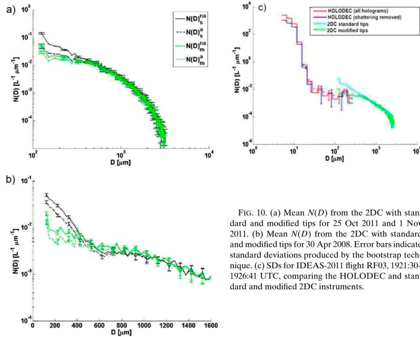
FIG. 10. (a) Mean  $N(D)$  from the 2DC with standard and modified tips for 25 Oct 2011 and 1 Nov 2011. (b) Mean  $N(D)$  from the 2DC with standard and modified tips for 30 Apr 2008. Error bars indicate standard deviations produced by the bootstrap technique. (c) SDs for IDEAS-2011 flight RF03, 1921:30–1926:41 UTC, comparing the HOLODEC and standard and modified 2DC instruments.
