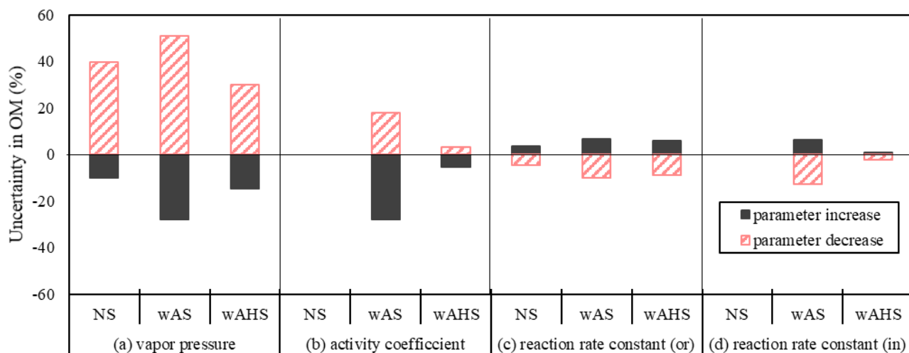
Figure 7. Uncertainties in UNIPAR-CB6r3 simulated gasoline SOA mass due to model parameters: (a) vapor pressure ( P_{L,i} ), (b) activity coefficient in inorganic phase ( \gamma_{in} ), (c) aerosol phase reaction rate constant in organic phase ( k_o ), and (d) aqueous phase reaction rate constant ( k_{AC} ). The errors associated with P_{L,i} , k_{AC} , and k_o were estimated by increasing and decreasing the factors by 150 and 50%. The uncertainties associated with \gamma_{in} were estimated through increasing and decreasing \gamma_{in} by 200 and 50%, respectively. The SOA formation was simulated at the high \text{NO}_x level ( \text{HC}/\text{NO}_x = 3 ppbC/ppb) under the given reference conditions (298K, 60% RH, and 1500 ppbC of gasoline vapor) under the specific sunlight intensity measured on 06/19/2015 (Fig. S5(a)). The concentration of pre-existing organic matter and inorganic seed was 3 \mu\text{g m}^{-3} and 10 \mu\text{g m}^{-3} , respectively.
