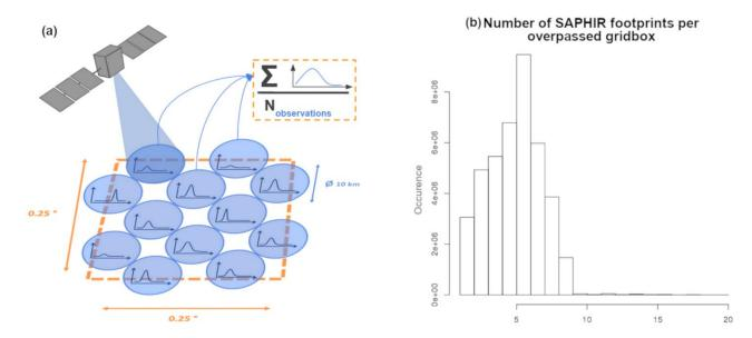
Figure 1: (a) Colocalization diagram of SAPHIR's PDF and ARPEGE grid and (b) distribution of the sample size of SAPHIR footprints in ARPEGE gridboxes.
