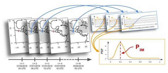
Figure 3: Diagram presenting the spatial and temporal aggregation method for a single grid point (blue square when the gridbox was passed over by SAPHIR, red when not and/or filtered out).  $P_{3M}$  is the mode of the distribution aggregated over all the considered time steps for this gridbox.
