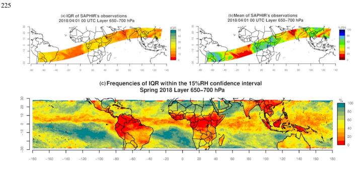
Figure 4: (a) Spatial distribution of the inter-quartile range (IQR) and (b) mean of reference ( $\overline{RH_{obs}}$ ) representing the observed spatial field of RH from SAPHIR on 01/04/2018 at 00UTC and at the 650-700 hPa layer (c) Frequency of  $IQR \leq 15$  %RH over the three-month period (April to June 2018)
