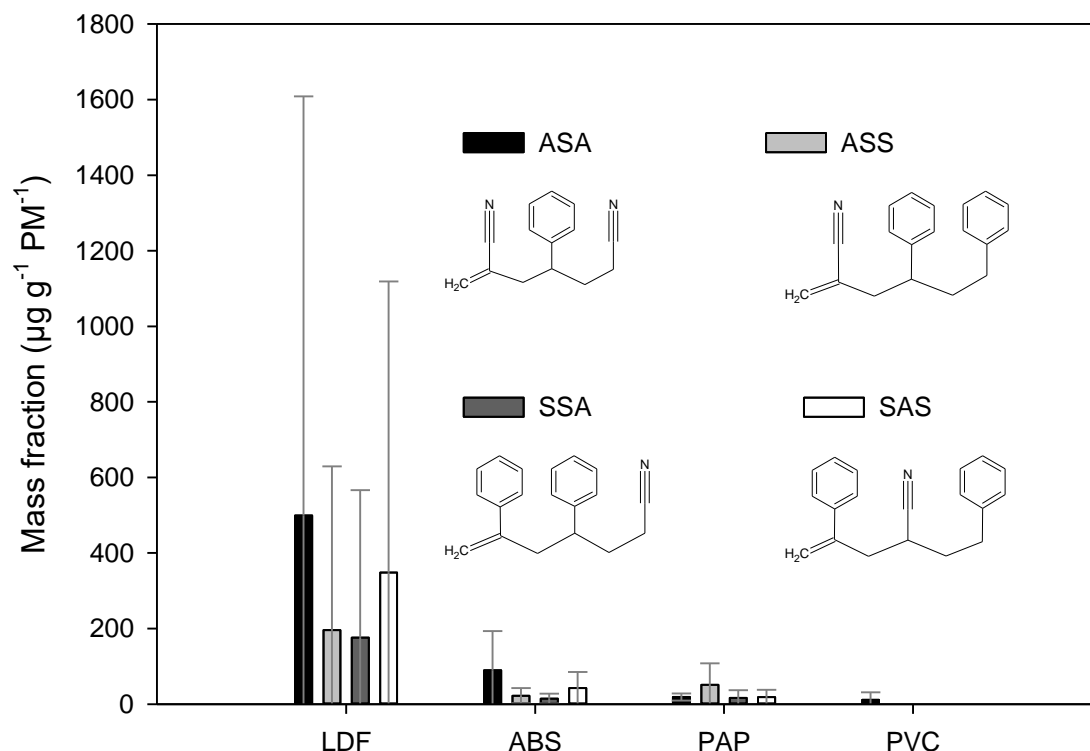
Figure 3 The mass fraction of the compounds (in units of \mu\text{g g}^{-1} \text{PM}^{-1} ) emitted during the burning of styrene containing copolymers. The error bars represent the standard deviation of the EF data obtained for a given type of waste under different burning conditions.
