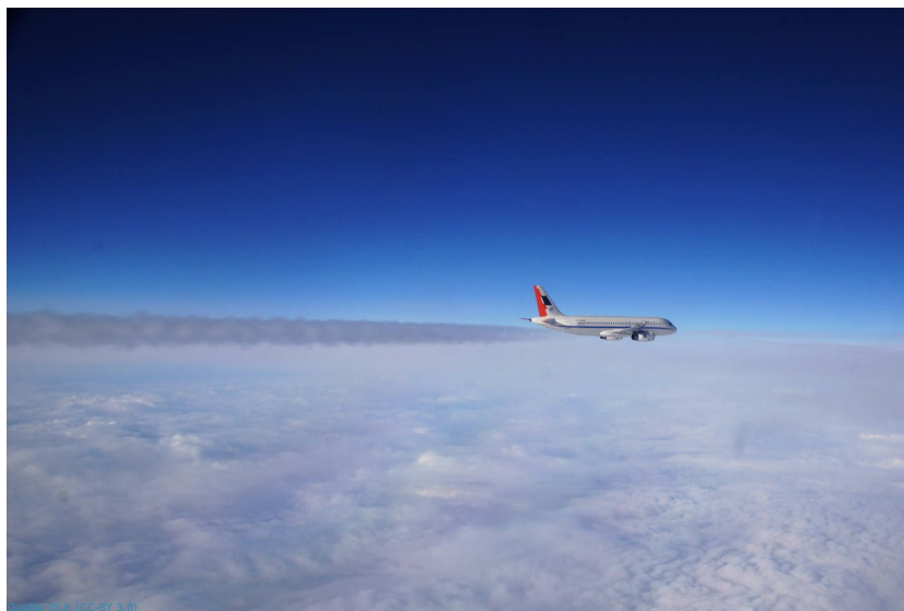
Figure 1. Photograph of the DLR A320 with contrail in January 2018 during the ECLIF II/NDMAX flight experiment.
