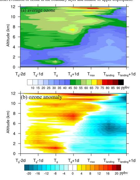
Figure 5: (a) Vertical ozone concentrations (unit: ppbv) at each typhoon developmental stage averaged over the typhoon ensemble over 2014-2018 at Taiwan. (b) Anomaly of vertical ozone concentrations relative to Tg-2d stage of the subsequent typhoon developmental stages. The temporally dense ozone profiles are available from the airborne observations of atmospheric compositions under the IAGOS framework collected at Taoyuan International Airport of Taiwan.
