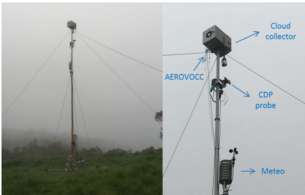
Figure 1. Location of Piste Omega and other instrumented sampling sites at Reunion Island. Photo of the mast (10 m height) deployed during the BIO-MAÏDO project integrating the cloud water collector, cloud droplet probe (“CDP probe”), meteorological station (“Meteo”) and gas phase collection (“AEROVOCC”).
