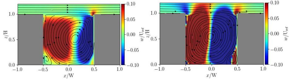
**Figure 1:** Spanwise-averaged vertical streamlines for a bottom-heated unit-aspect-ratio street canyon and an external wind perpendicular to the canyon axis (Wang et al. 2021). (a) Neutral flow ( $Rb=0$ ); (b) Unstable flow ( $Rb=-0.39$ ).
