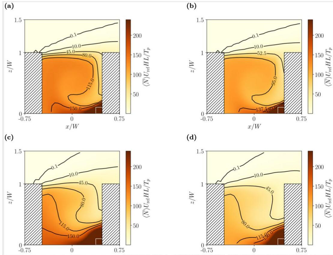
**Figure 2:** Comparison of results for different wind directions with respect to the axis of unit-aspect-ratio street canyon: (top) perpendicular ( $\theta=0^\circ$ ); (bottom) parallel ( $\theta=90^\circ$ ). (a,c) without microphysical processes; (b,d) with microphysical processes.
