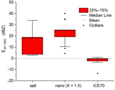
545 Figure 10: The box and whisker plots presenting the efficiency range of three different seeding materials. The box plots are evaluated from data representing different background aerosol types and different updraft velocities.
