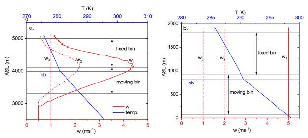
Figure 1: The temperature profiles and the prescribed updraft profiles in the numerical simulation for (a) the SPEC UAE cases and (b) the QCSRP cases. The horizontal blue lines denote the altitude of the cloud base. The three horizontal black lines from bottom to top denote the level where the calculation of the diffusional growth starts (RH = 70%), the levels 100 m and 1000 m above the cloud base.
