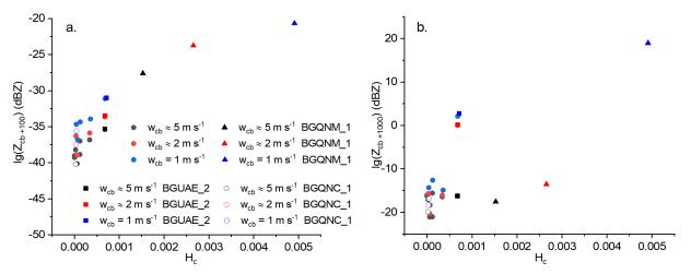
Figure 3: Reflectivity calculated from the modelled DSD (a) 100 m and (b) 1000 m above the cloud base for non-seeded control cases. Symbols with different colours represent different updraft velocities at the cloud base as indicated by the key. Sensitivity on the updraft velocity in the case three different background aerosol size distributions is presented by different symbols (see the legend in panel a.).
