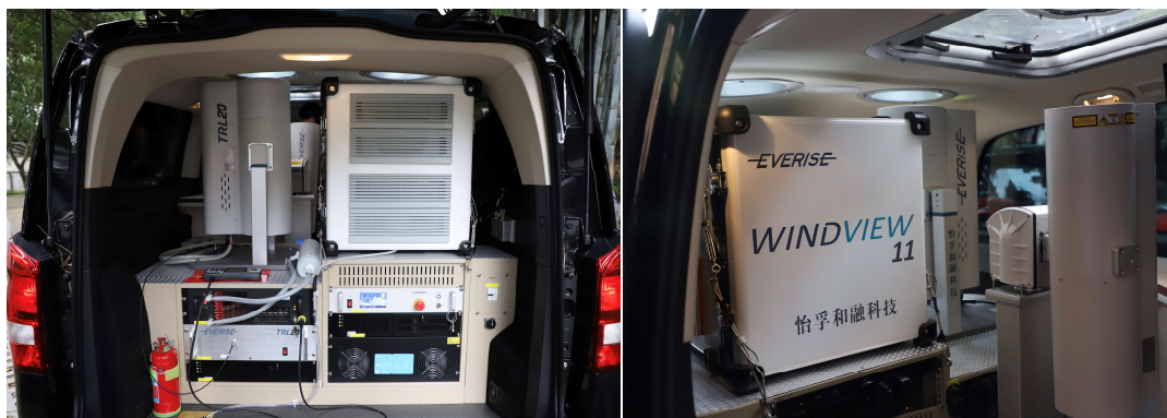
137 Figure 2. Setup of the multi-lidar system on the vehicle.
