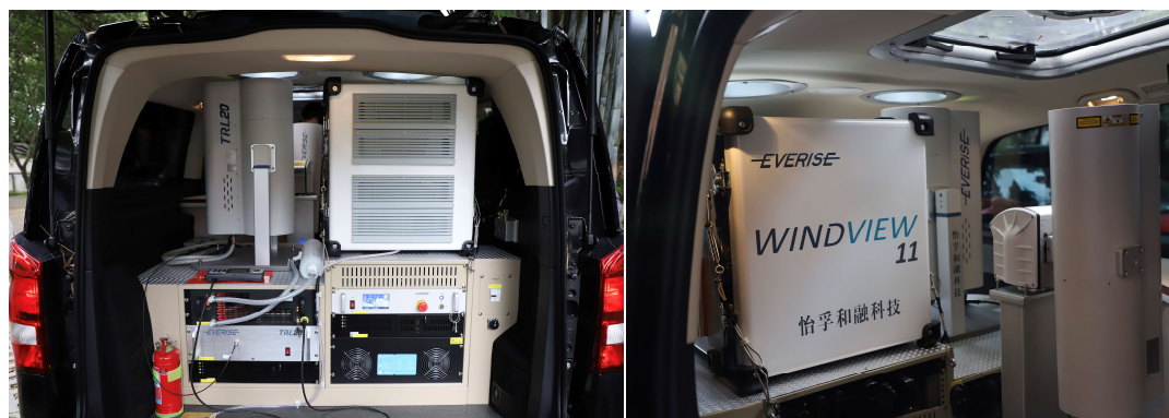
Figure 2. Setup of the multi-lidar system on the vehicle.
