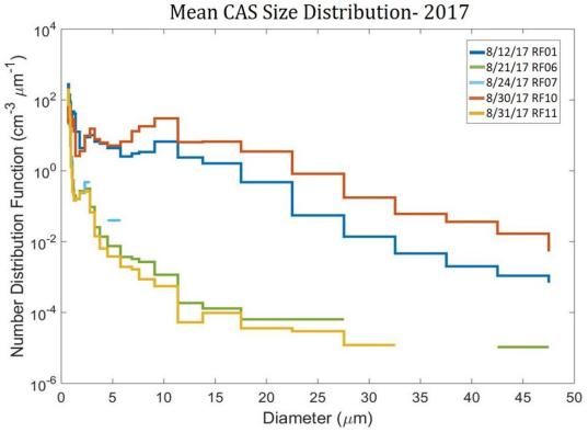
**Figure 4.** Mean cloud and aerosol spectrometer (CAS) aerosol size distribution for five research flights during a five minute interval when 2D-S SAPs were measured within the BB plume.
