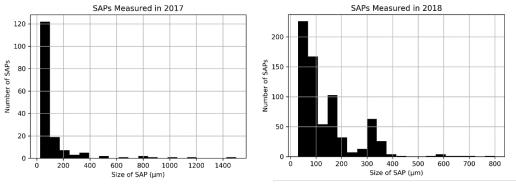
**Figure 12.** Particle sizes for the 165 SAPs measured in 2017 and the 692 measured in 2018.
