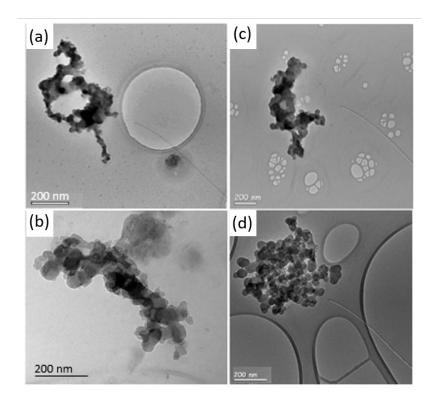
**Figure 6.** Transmission electron microscope/microscopy (TEM) images of black carbon particle aggregates collected on August 30<sup>th</sup>, 2017 (A), August 31<sup>st</sup>, 2017 (B), October 2<sup>nd</sup>, 2018 (C), and October 3<sup>rd</sup>, 2018 (D) on gold grid polycarbonate filters.
