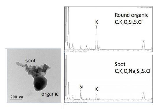
Figure 7. Energy-Dispersive X-ray Spectroscopy (EDS) elemental analysis of an organic/soot particle from RF 11, August 30<sup>th</sup>, 2017.
