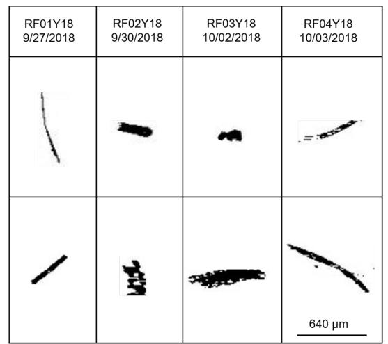
**Figure 8.** SAPs recorded within the BB plume by the 2D-S probe during the ORACLES 2018 campaign. SAPs were observed to be a variety of size and shapes ranging from 10-1000 μm in length.
