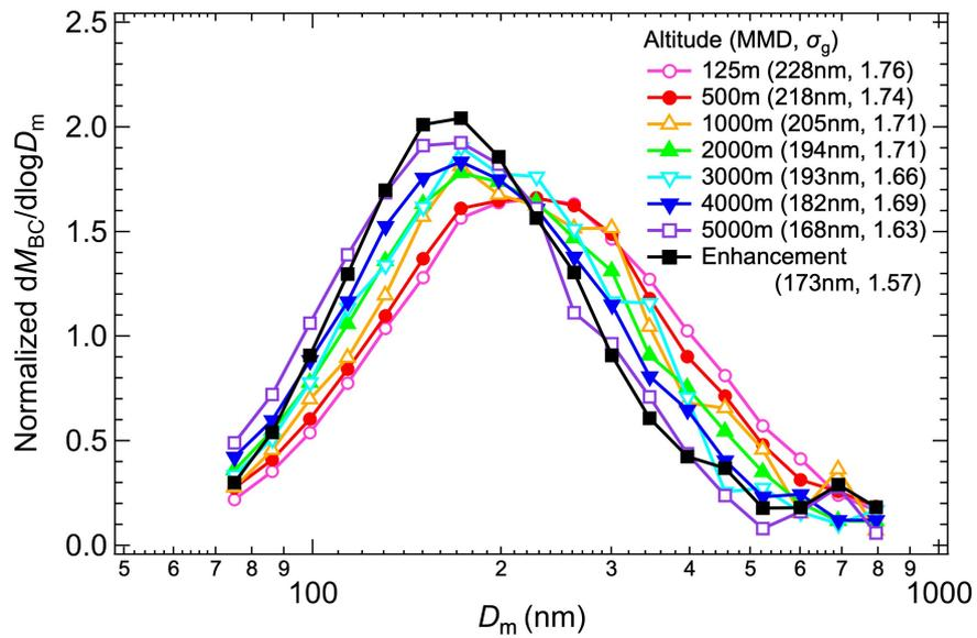
**Figure 9.** Averaged mass size distribution of BC in each altitude range. Values normalized by the total mass concentrations of BC ( $(dM_{BC}/d\log D_m)/M_{BC}$ ) are shown. The average size distribution for the enhanced  $M_{BC}$  data is shown with black squares. The numbers shown in parentheses are the mass median diameter (MMD) and the geometric standard deviation ( $\sigma_g$ ) for the lognormal fitted size distributions.
