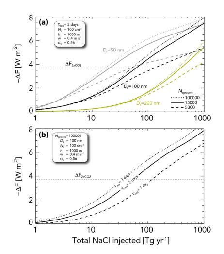
Figure 6: Radiative forcing as a function of the total (global) rate of salt mass injection, for (a) three sprayer numbers ( $N_{sprayers}$ =5300, 15000, and 120000), and for geometric mean spray diameters  $D_s$  of 50 nm (gray), 100 nm (black), and 200 nm (yellow); (b) forcing for  $N_{sprayers}$ =120000 and  $D_s$ =100 nm as a function of injected particle lifetime. All other parameters are the same as those used in Fig. 5.
