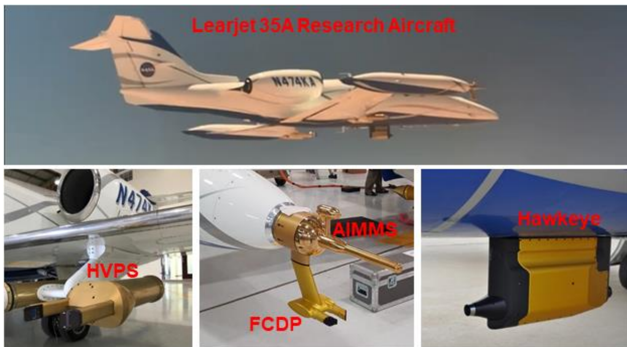
Figure 4. Learjet in-flight over Al Ain and selected instruments: HVPS, FCDP, AIMMS and Hawkeye (from left to right).
